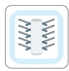
Electronic Membrane Life Enhancer - EMLE Prevents scaling of dissolved salts like calcium and magnesium, thereby enhancing the membrane life and improving water flow.
